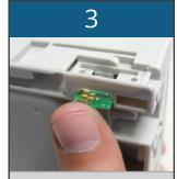
Insert the original chip into the new compatible ink cartridge as per the diagram.
