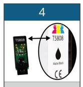
Check that the code on the ink cartridge matches the code on the added supplier chip.
